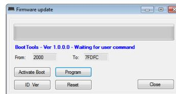
The updating of **WEBS** module does not need any address, therefore click on the button "**Activate Boot**" and then "**Program**" to start updating; at the end, the program will wait for the reinitialization of **WEBS** (10 seconds about), then the new firmware version and the IP address of the module will be shown. The button "**ID Ver**" allows to check the ID code and the firmware version; the button "**Reset**" allow resetting the module (if needed).
