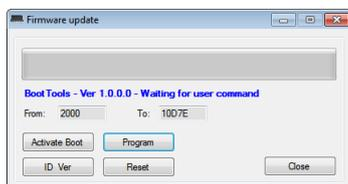
The updating of FXPRO2 does not need any address, therefore click on the button “**Activate Boot**”: the display of FXPRO2 will show “Firmware Updating”; click then “**Program**” to start updating; at the end, the program will automatically reset FXPRO2.
