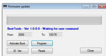
The updating of *DFGSM3* module does not need any address, therefore click on the button “*Activate Boot*” and then “*Program*” to start updating; at the end, the program will automatically reset the module.
