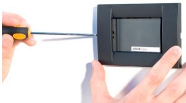
Release the module from the frame by inserting a screwdriver on the central hook (\*\*).
