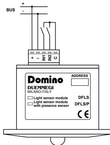
In the case of -P version, IN2 input can be connected to an additional presence sensor which must operate in parallel with the built-in sensor; for the **DUEMMEGI** SRP sensor the wiring is the following:
