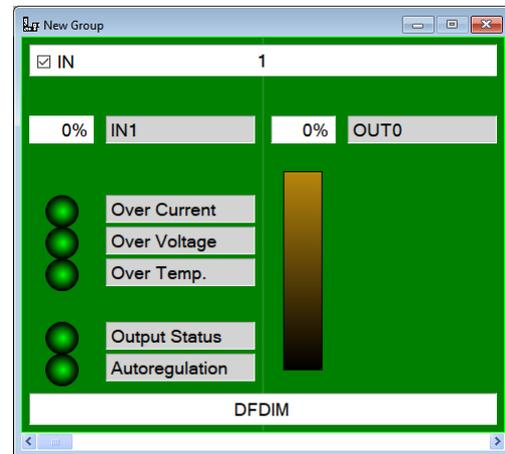
As for all **Domino** modules, the background of the module is in green color if the module is connected and properly working, otherwise the background is in red color.
